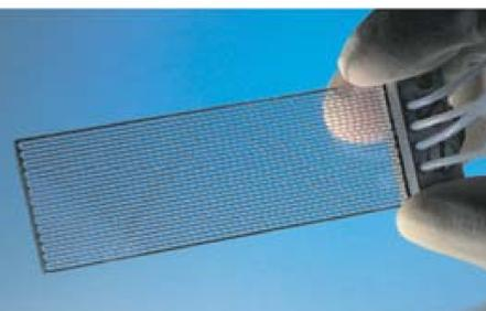
Fig.5: Picture of the all-glass prototype of the fluidic module with fluidic interface
